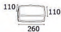
LW 30332 W260 x H110 x D110 mm LED Aluminum CE, RoHS, IP65, ENEC
