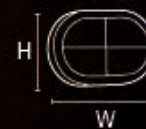
LW 30341A/B/C A-W214 x H130 x D64mm B-W275 x H180 x D100mm C-W340 x H210 x D108mm LED / E27 x 1 Aluminum CE, RoHS, IP65, ENEC
